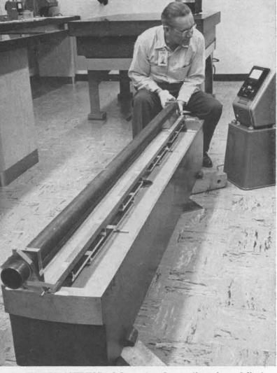
PRECISE MEASURING of large foundry castings is a delicate matter. Here J. M. Bunch (1651-2) takes a meter reading after carefully aligning gauge blocks along the length of the casting. Sandia is one of 20 selected firms participating in a project for the National Bureau of Standards and American Ordnance Association.
